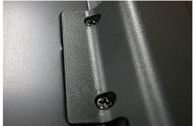
4. Lock the screw to mount MSR
