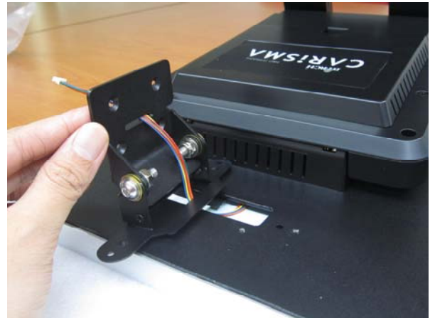
7. Pass the signal line through the middle of the lower hinge mount hole
