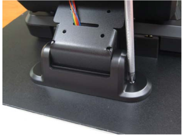
17. Lock the hinge cover by screw
