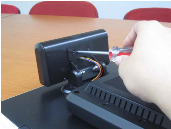
18. Lock the VFD module with hinge mount
