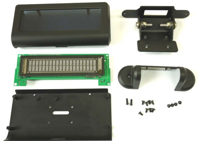
3. Release the screws on the VFD module
