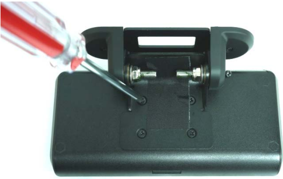
1. Release Four screw on the back of VFD module
