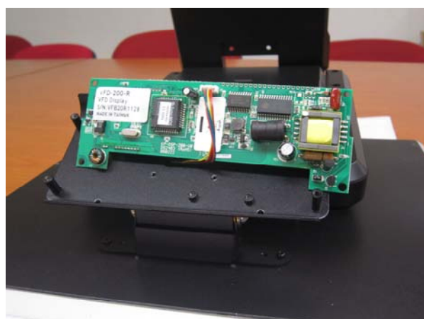
11. Connect the signal line with VFD board
