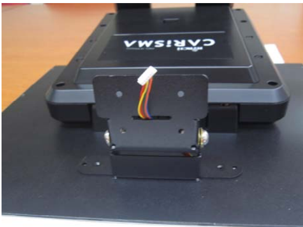
8. Pass the signal line through the middle of the upper of hinge mount hole
