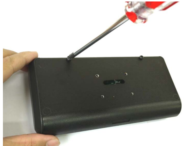
3. Release the screws on the VFD module
