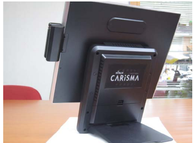
4. Lock the screw to mount MSR
