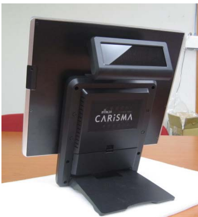
18. Lock the VFD module with hinge mount
