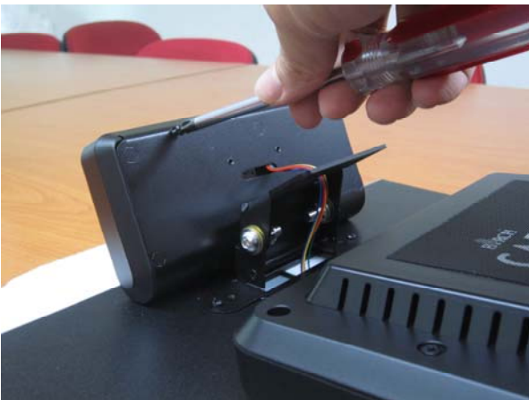
14. Lock the VFD cover with VFD base
