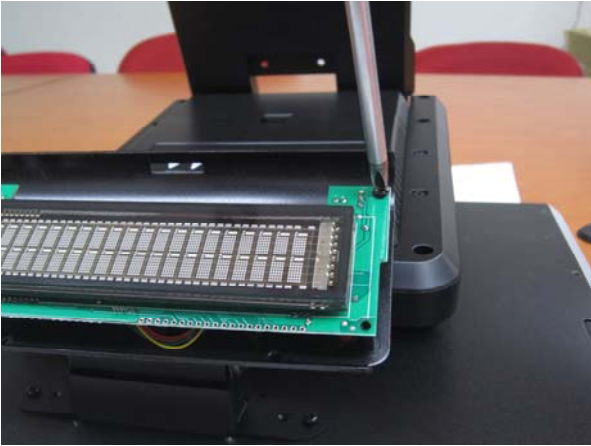
12. Lock the VFD board by screws
